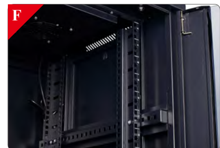
Front and rear sets of vertical rails adjust in quarter inch increments. Simply unscrew the rails, adjust them to the required depth and re-fasten.
